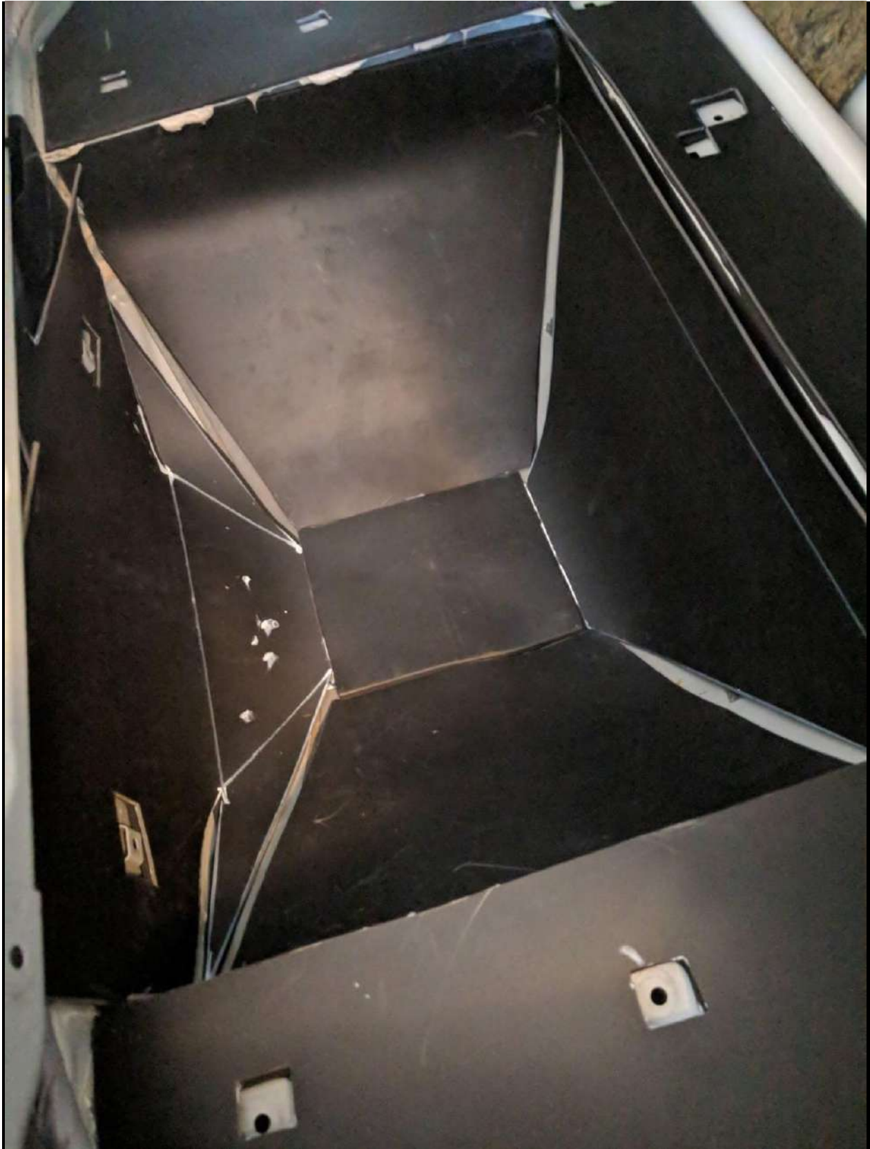
The back of the trunk and the trunk well are also treated with CCF and MLV
