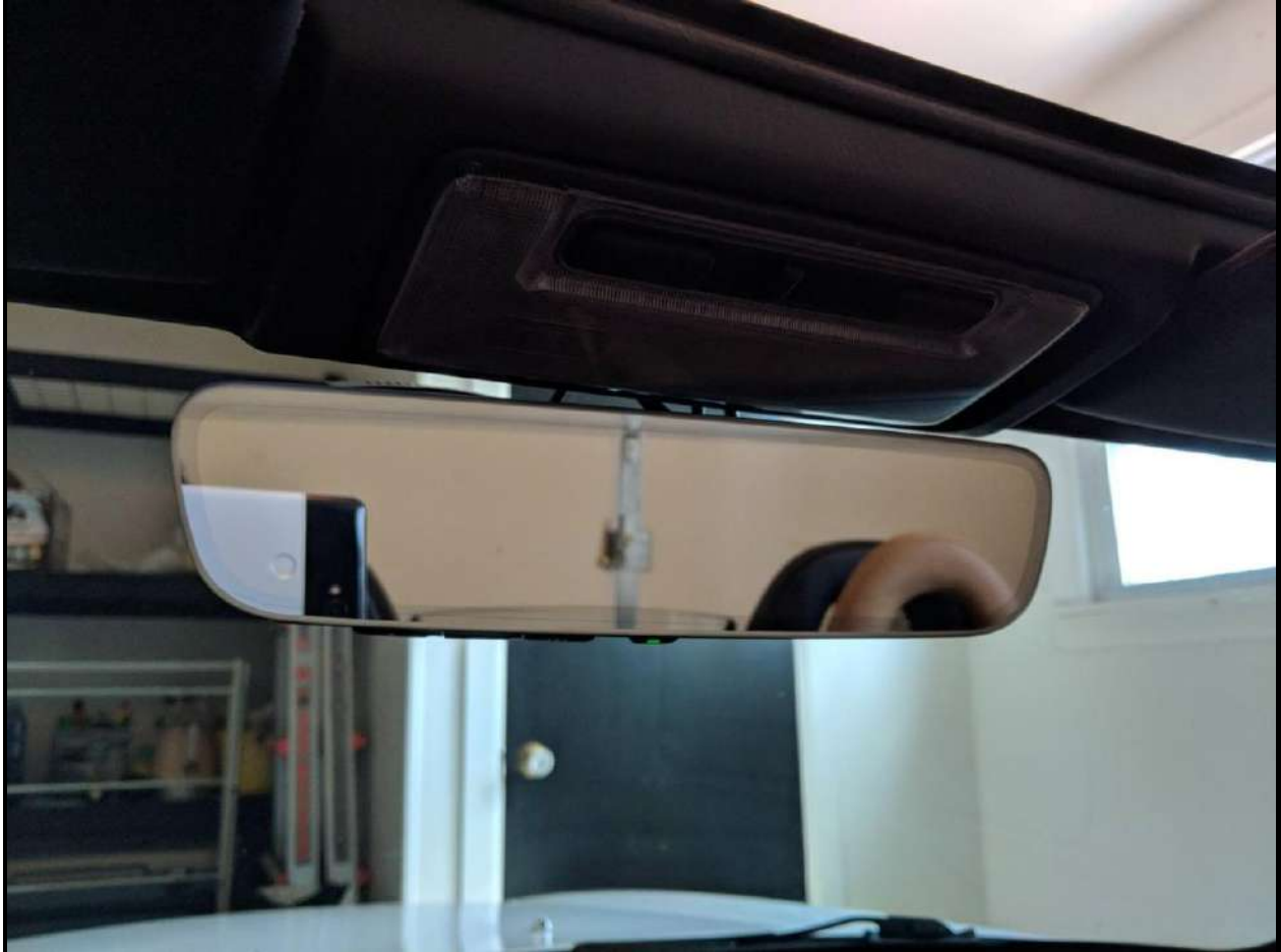
Here you can see the mirror as the driver would normally see it. It obscures the dash cam and EZ Pass tag well.
