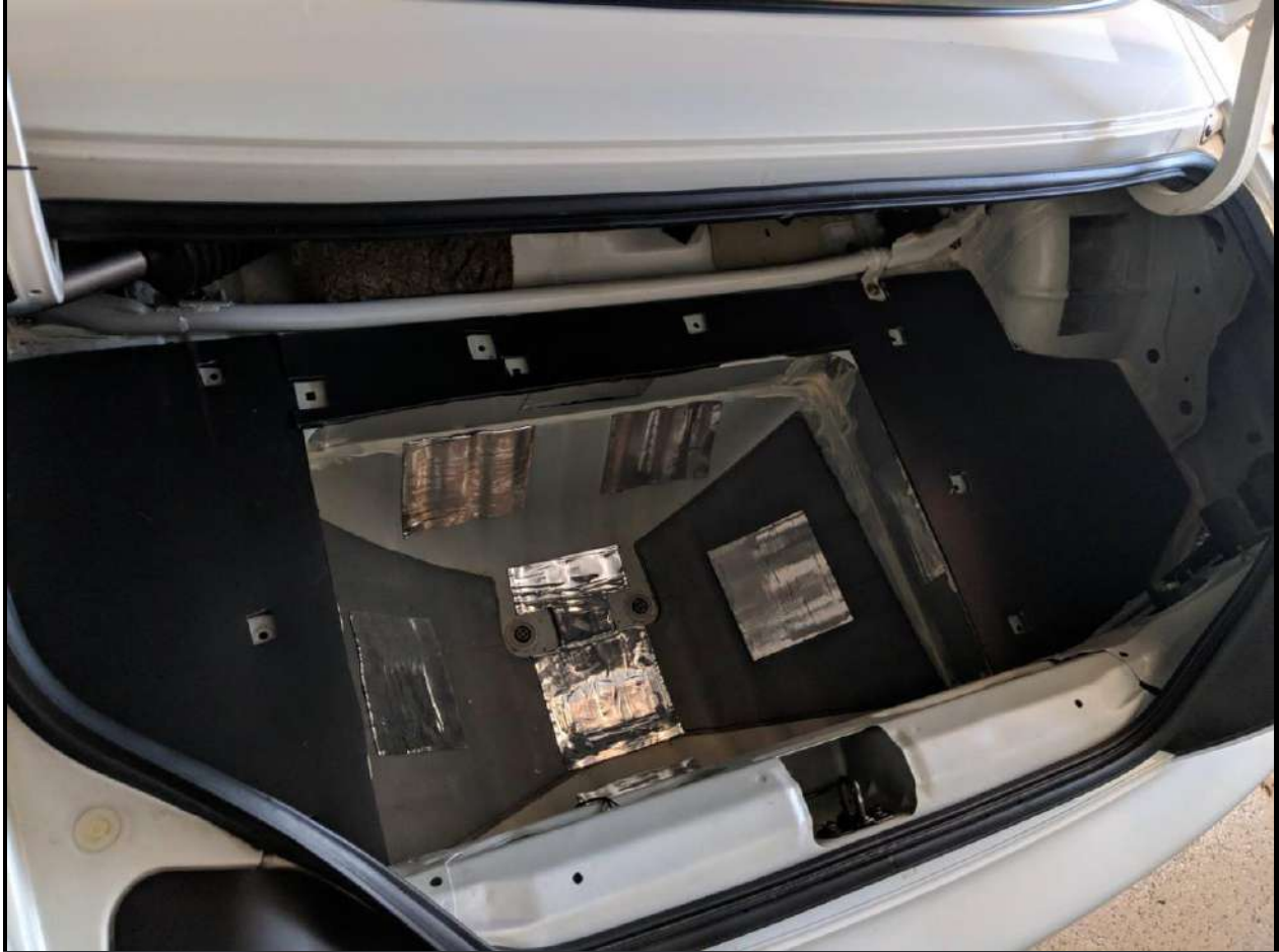
The floor of the trunk is treated with CCF and MLV, with holes cut out for mounting the trim panels
