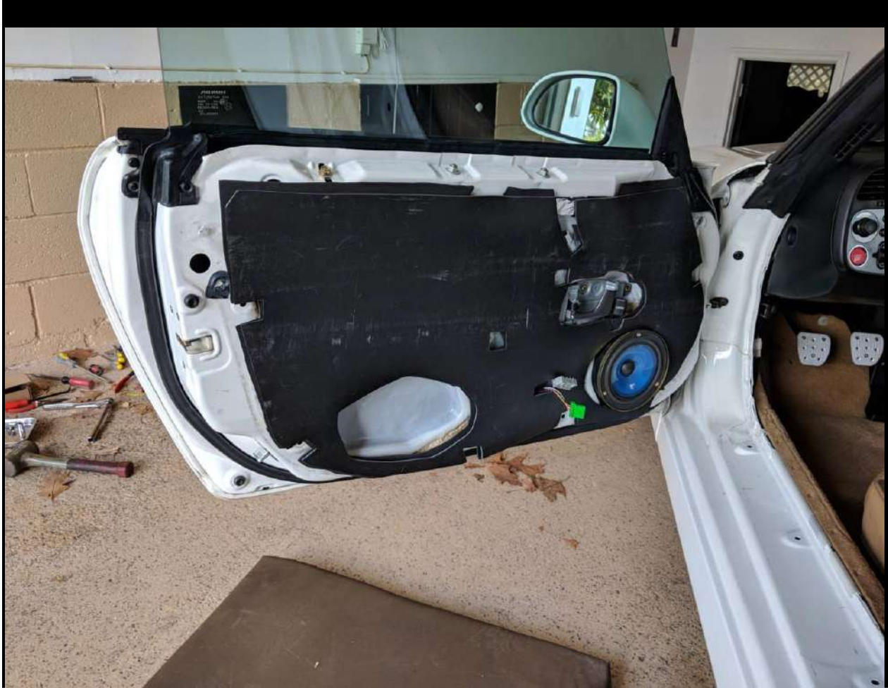
This is the first mockup for the driver's side door treatment. Both CCF and MLV are applied here
