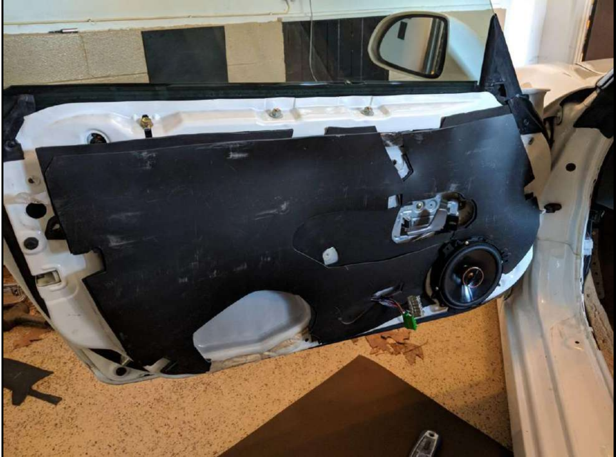
Some trimming was done to the CCF and MLV, to allow the door panel to sit properly on the door. A large center section had to be removed, as it was fouling the door latch/lock mechanism
