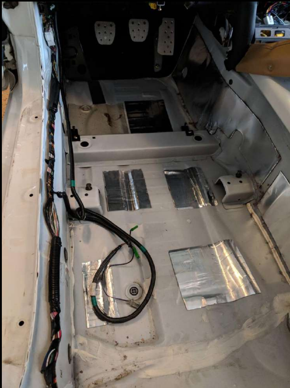
CDL tiles were applied to the driver's side floor. The kit from SDS has recommendations on how many tiles should be applied to each area.
