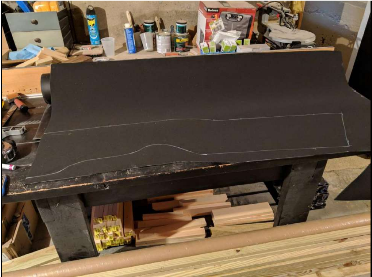
The CCF for the passenger's side of the center tunnel is measured and traced out. From here it is cut out and then trimmed to fit. Once it fits properly, the size is transferred to MLV, for a matching piece.
