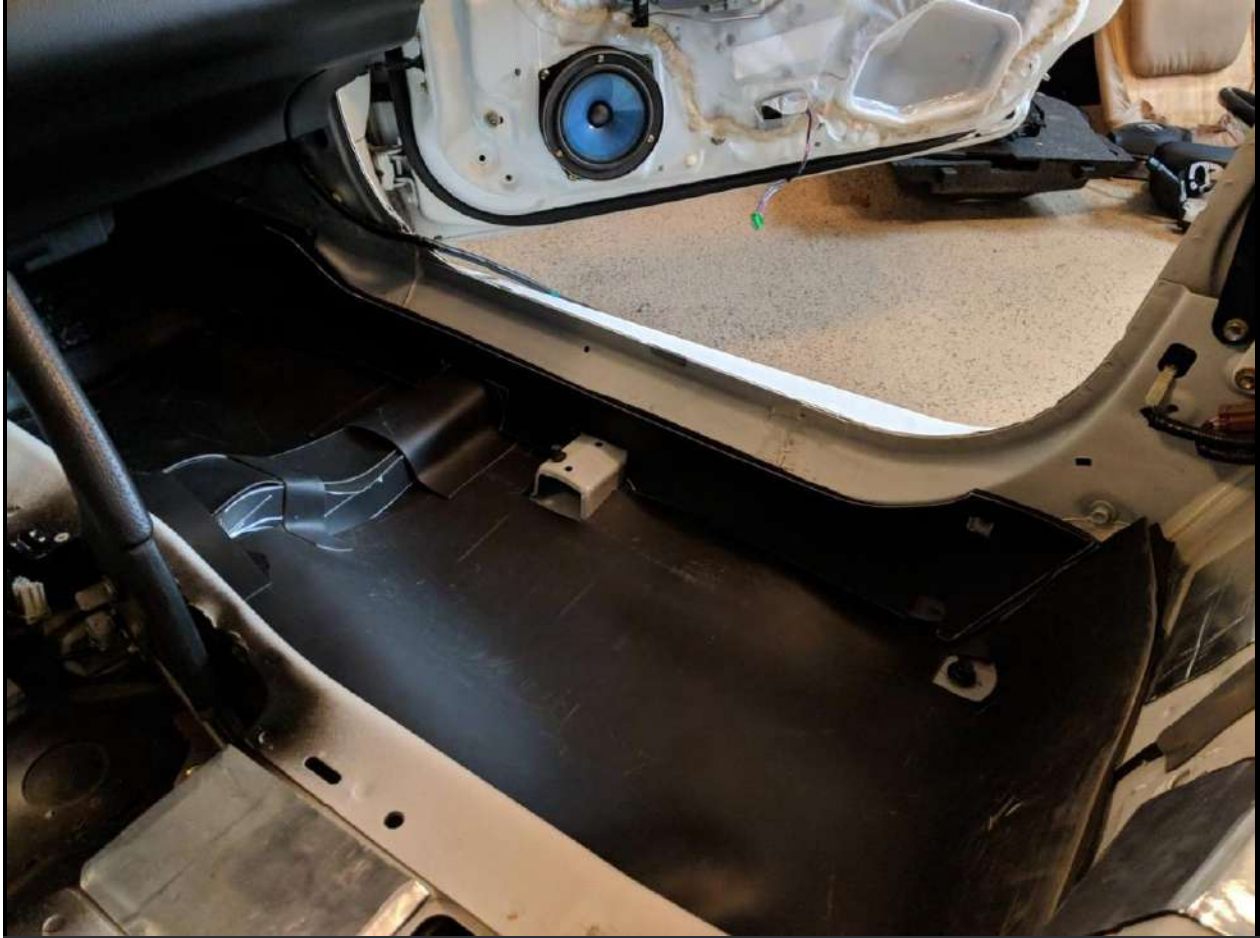
The passenger's side kick panel and under door area is treated with CCF and MLV
